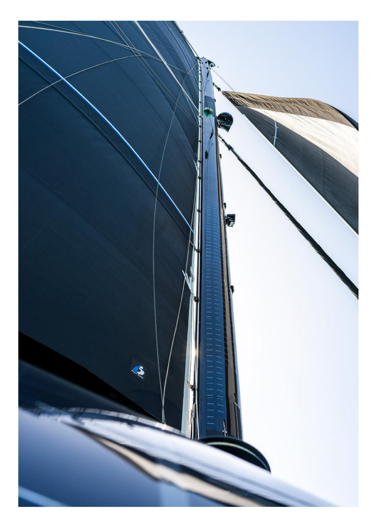
Thanks to the shipyard's award-winning technology the craft can welcome up to 242,5m² of composite-integrated solar panels, generating up to 45kWp.
